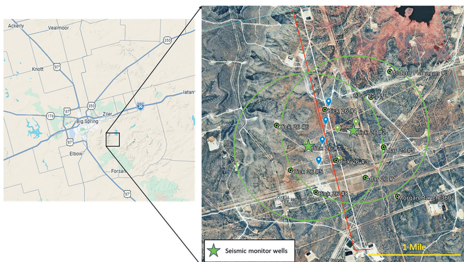
Figure 3. Area map for Howard County, Texas, showing the outline of the field experiment southeast of Big Spring at the Signal Peak field area. Green stars on the enlarged map denote the click 26 #2 and #7 wells that were used for observation wells in the experiment. Blue and green markers show the locations of the SensorEra surface stations. Green circles represent the expected 4000 ft radius of detection limits for microseismic events for both observation wells. The red and white lines are the well trajectories for the MCC wells.
