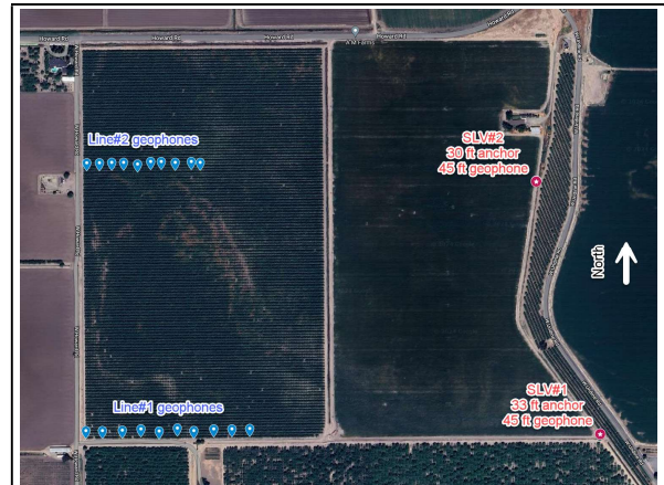
Figure 1a: Map view of acquisition. The test field is near Stockton, California. SLV sources in red pins and sparse surface receivers in blue pins.
