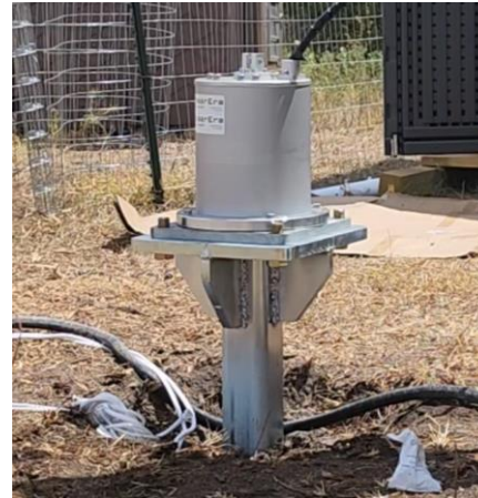
Coupled with Earth All vibrations pass through (Houston Test Site) 4,200lb version
