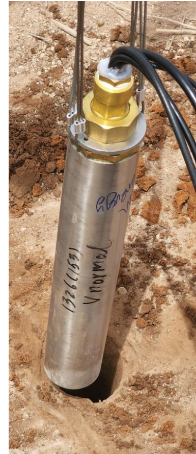
New 6C motion + 3C orientation MEMS seismic sensor sonde being deployed (1.9" diameter)
