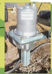
Remotely Controlled Solar Seismic Sources, below weathering layer
