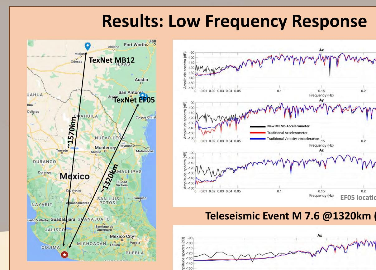
A M7.6 earthquake occurred over 1000km from the sensors in Texas, which was detected by TexNet seismometers and the new MEMS stations. The data demonstrated a
