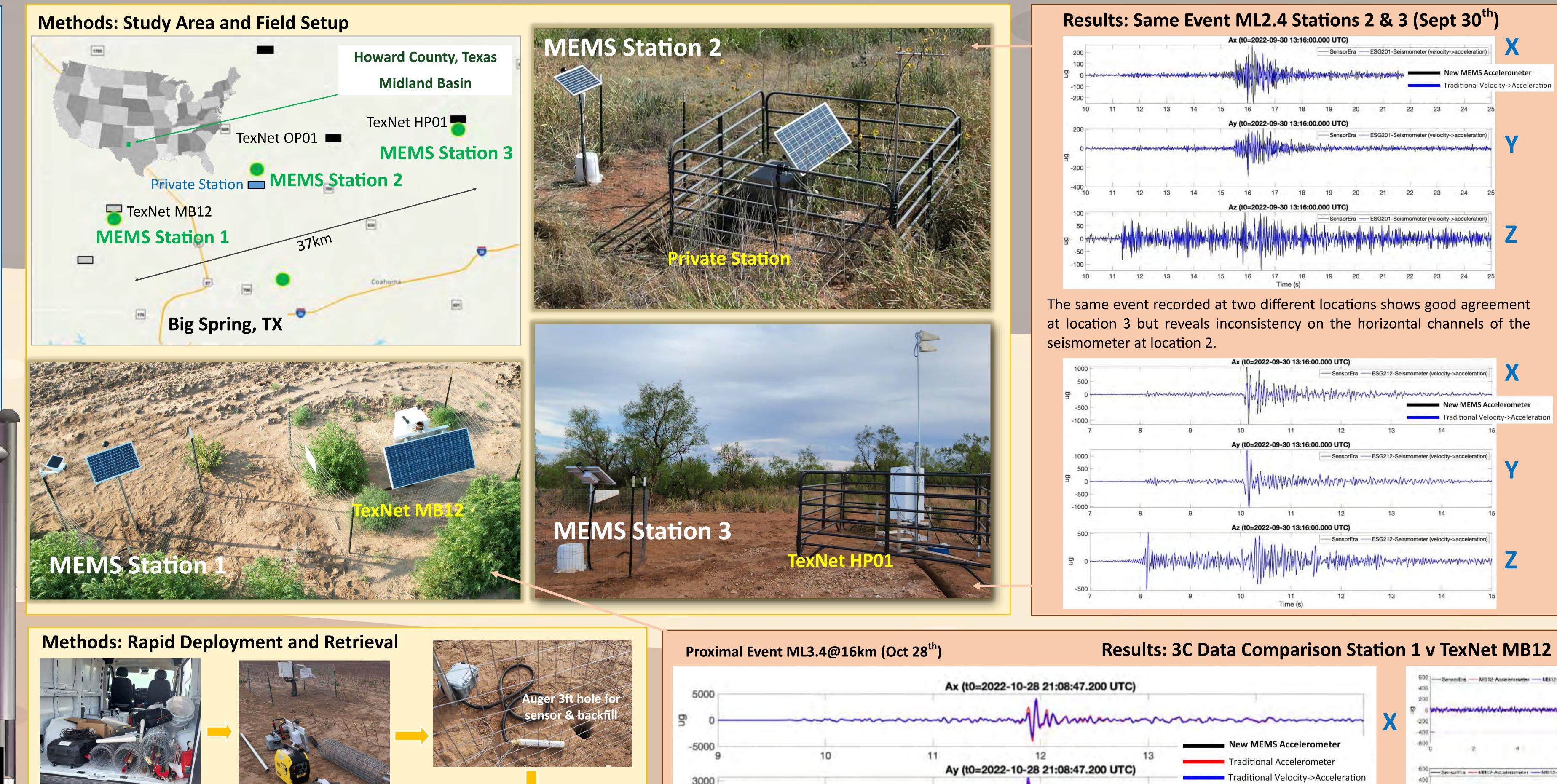
Sensor stations can be easily transported by road, with up to tens of stations per vehicle. Onsite installation involves making a 3-4ft hole for the sensors and setting up charging and communications masts using only handheld equipment. Installation time including cattle fence is 1-2 hours and removal time is 1 hour. The new MEMS sensors are self-oriented by on-board magnetometer and require no settling time to begin recording immediately.
