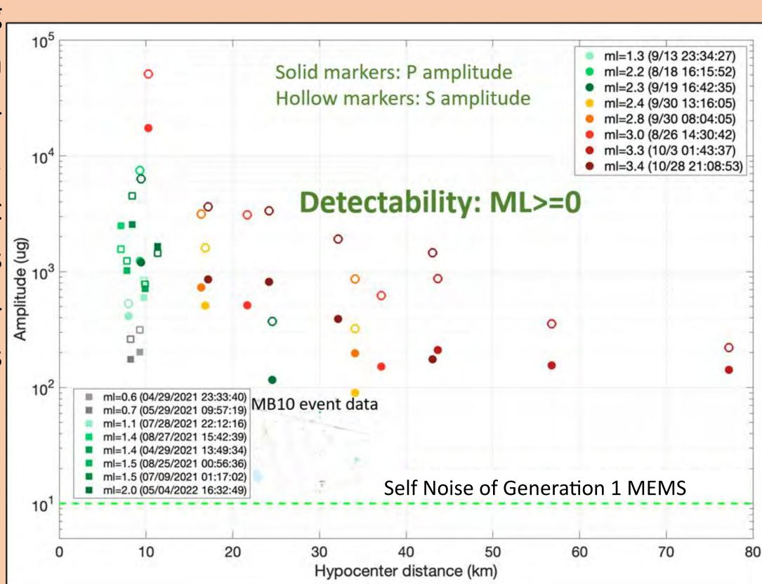
The traditional seismometers show a minimum amplitude of approximately 100µg, while stronger events seen nearly 80km away show ML between 3-4. The MEMS sensors, with a self-noise amplitude of 8-10µg (recently upgraded to 1ug), are suitable for monitoring in this area as this is well below the smallest recorded signal amplitude.
