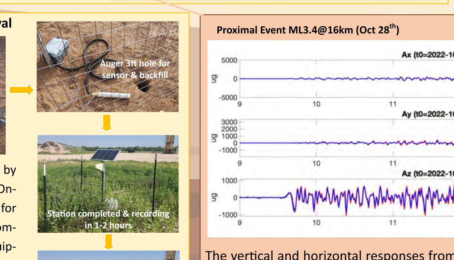
Station removed in 1 hour, zero
