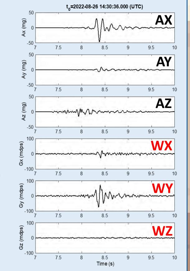
The sensors measure 3-component translational motion and 3-component rotation. When there is strong motion, such as a 2.7km ML 3 quake close by, the response can be seen on all six components.
