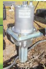
Remotely Controlled Solar Seismic Sources, below weathering layer
