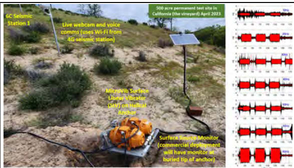
Figure 5: The SLV source installed on a helical anchor at the SensorEra/GPUSA 500 acre test facility in California (the vineyard) April 2023. A series of tests were performed at discrete frequency bands and amplitudes were observed at the surface sensor. After correlation reflected energy was seen at 7000ft depth. Testing is ongoing.
